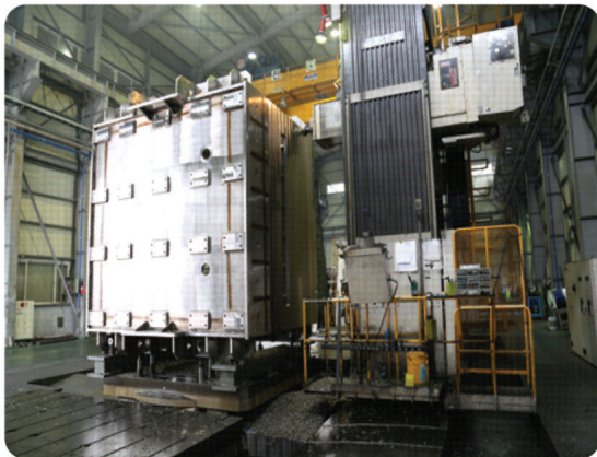
CNC Boring (X10000*Y4000*W2000)
