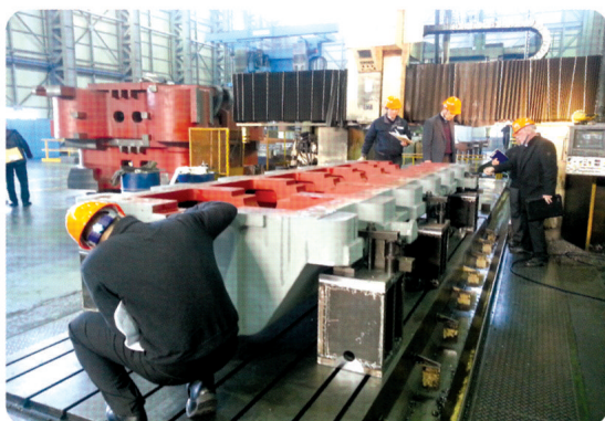
Compressor base plate inspection / 检查压缩机底盘
