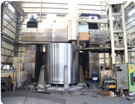
Vertical Turning Center M/C ( \Phi 6620 *W3700(H))
