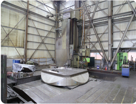
CNC Floor Boring (X6000*Y3200*W1450)
