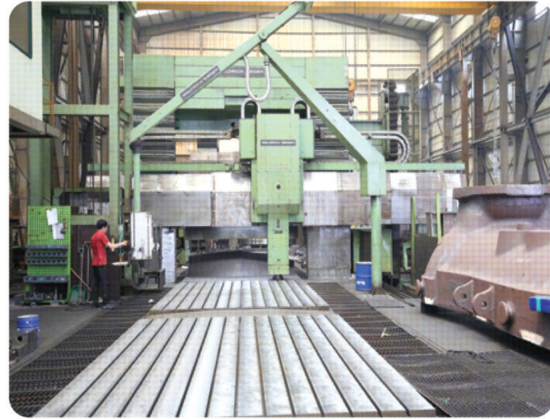
CNC Plano Miller (X12000*Y4000*W3000)
